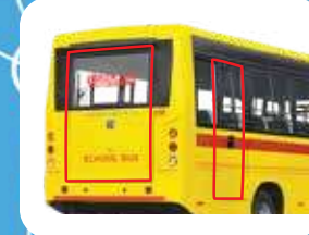
Two Emergency Doors
