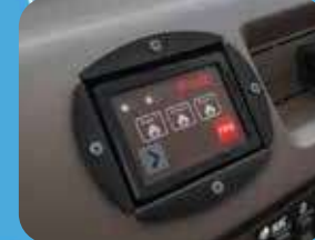
Fire Detection and Suppression System*
